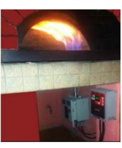
This new burner works like classics new Sputafuoco electromechanical generation, but much quieter, performing and efficient. Two flame lengths predetermined, minimum and maximum, with automatic control temperature. Possibility to choose instantly if use the minimum flame, the maximum flame or automatic control temperature, simply by pressing the reference button. The thermal power is 25 KW
